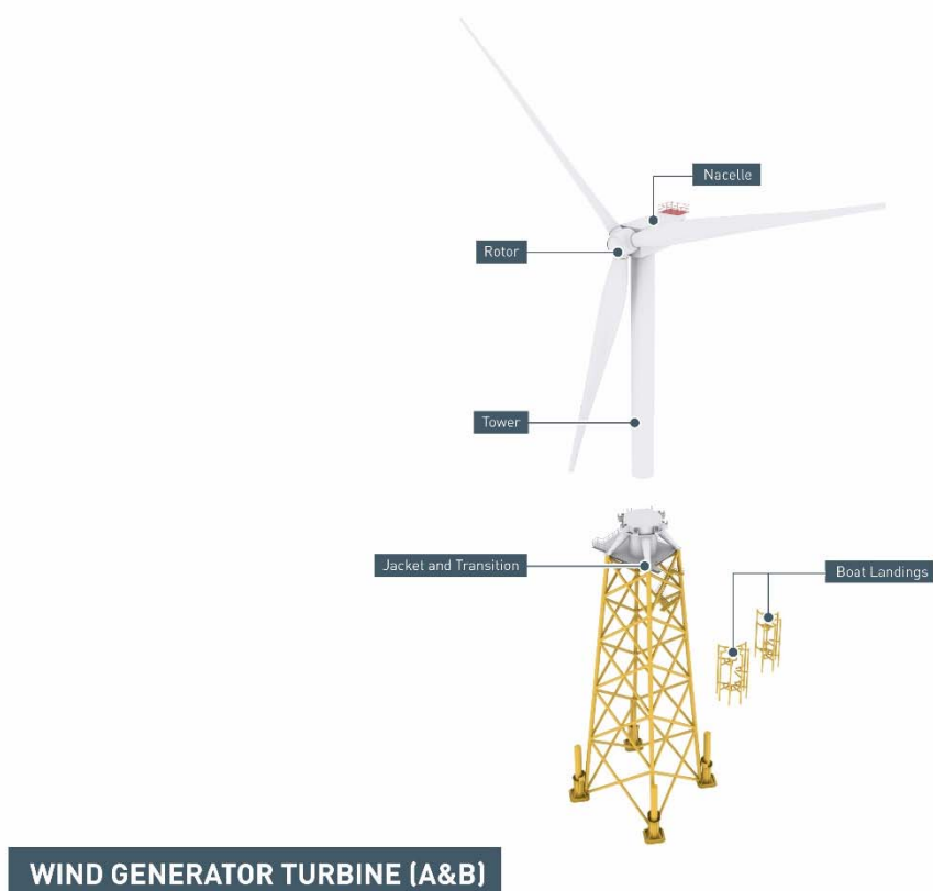
Figure 3.9: Beatrice Wind Turbines Schematic Showing Exploded View
